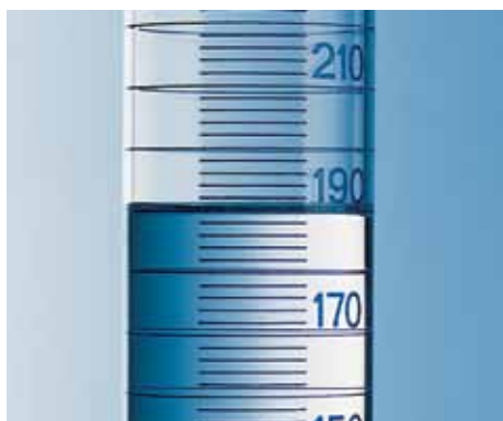
BLAUBRAND®. Ring marks at major graduations. Reading at lowest point of meniscus.
